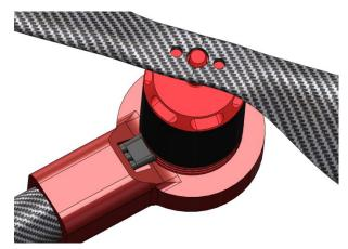
In order to have modifiable design motor holders are easily changeable and suitable for every kind of motor.
