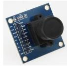
functions, including exposure control, gamma, white balance, color saturation, hue control and more, are also programmable through the SCCB interface. In addition, OmniVision CAMERACHIPs use proprietary sensor technology to improve image quality by reducing or eliminating common lighting/electrical sources of image contamination, such as fixed pattern noise (FPN), smearing, blooming, etc., to produce a clean, fully stable color image.
