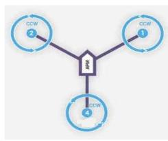
Tricopters has 3 motors that are usually 120 degrees apart and generally in Y configuration. Two propellers at the front sides and other propeller at the rear center. Rear motor has a servo mechanism to enable yaw motion of the system.
