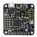
At the heart of the Naze32 is a 32bit ST micro work horse of a processor, with untapped memory and cpu power and a host of equally impressive sensors. The Naze is also matched up with some of the nicest GUI programs and features to get the most out of your configuration.
