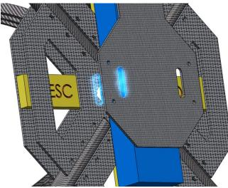
Plate's places where ESC's center is mounted is empty. The reason is cooling. Frame has openness at the front and air enters and circulation is completed through ESCs.
