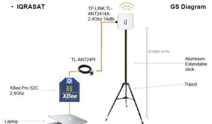
Fig. 13. The Ground Station Design
