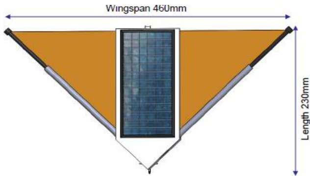
Fig. 1. Physical Layout of Science Glider
